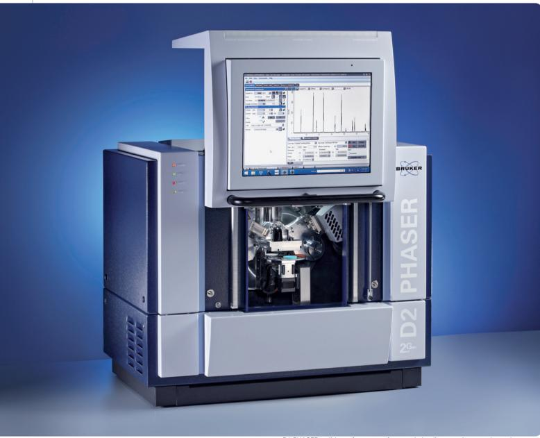
D2 PHASER – slide-up front cover for sample loading, monitor remains active
