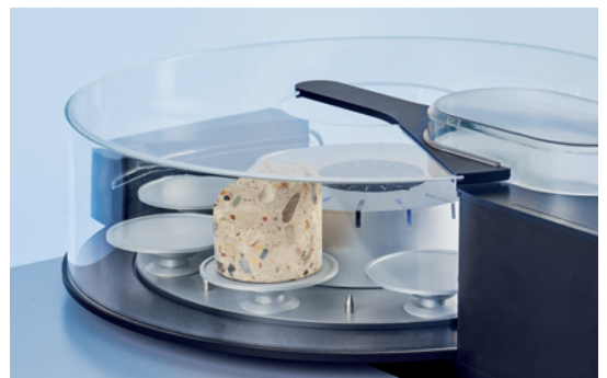
Up to 8 large samples (96 mm) or a random combination of large and small samples
