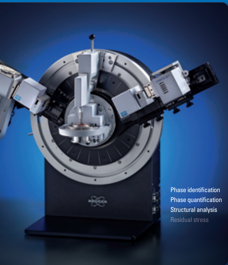
Bragg-Brentano geometry with energy-dispersive LYNXEYE XE-T detector and Motorized Anti-Scatter Screen
