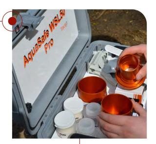
The Aquasafe Premium's and Pro's all include the HydroTest® HT1000 Multiparameter Photometer. The HT1000 is a compact but powerful handheld photometer which is lightweight and offers an easy colorimetric solution at the touch of a button using simple tablet reagents.
