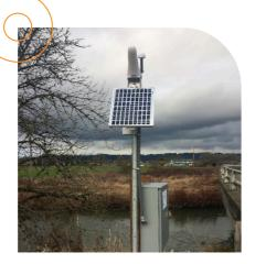
housed in secure cabinets, to protect from the elements and animal/human interference. The Maji-Stat is efficiently powered by both battery and solar panels, for minimum maintenance.
