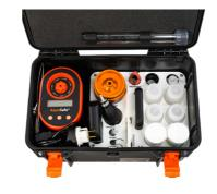
A small, yet extremely rugged, case allows this water safety kit to be carried anywhere with no concerns about user fatigue or space. Once opened, the kit allows simple, accurate and efficient testing of all the key water safety parameters including pH, conductivity, chlorine, ammonia, nitrate and nitrite, total arsenic, temperature, turbidity and faecal (thermotolerant) coliforms.
